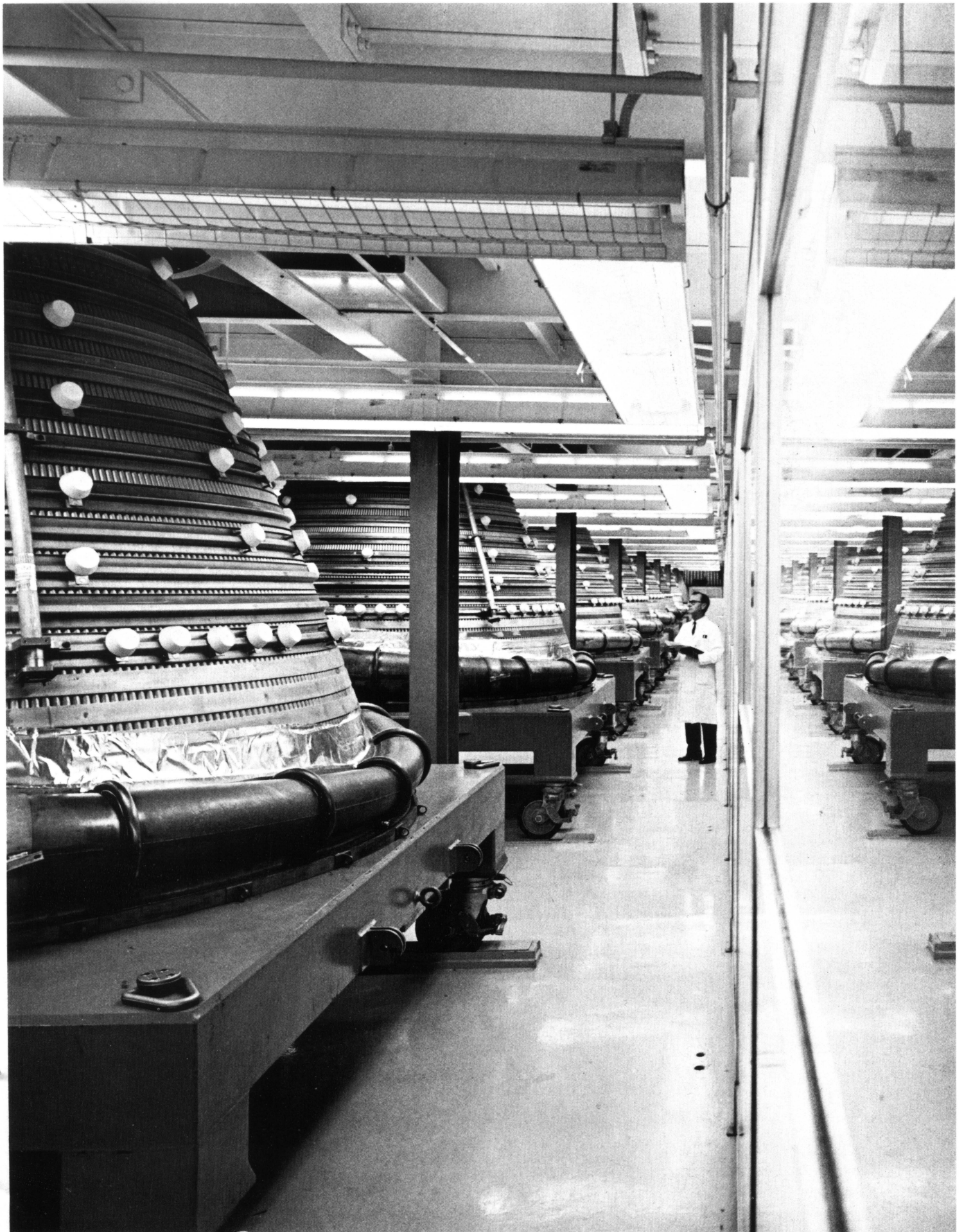
Five of these Rocketdyne F-1 engines, with total of 7,500,000 pounds thrust, lift entire weight of Apollo 4. In 1640 engine test starts, there has not been a failure due to engine hardware.
