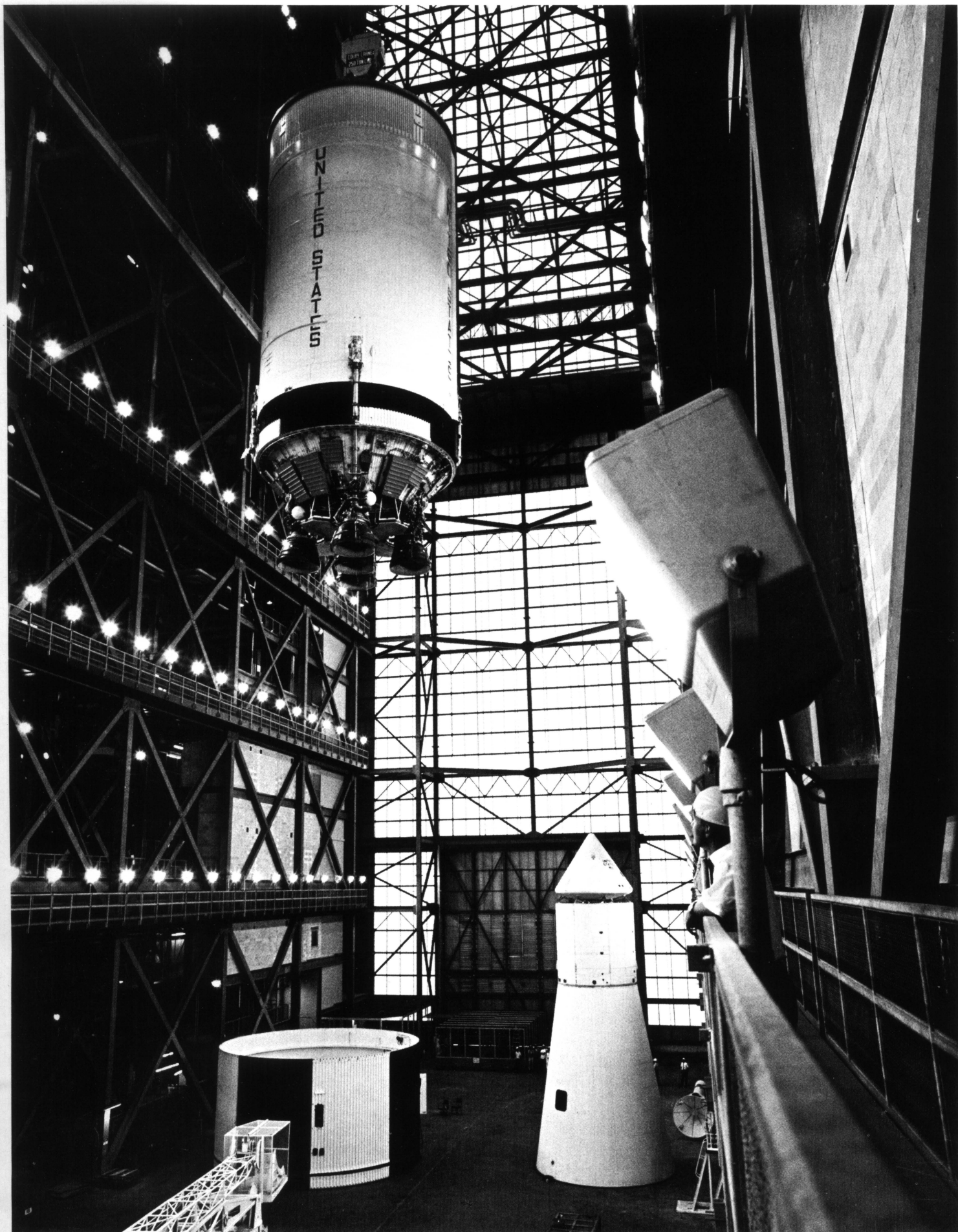
At Kennedy Space Center, Fla., months of final preparation precede the moon vehicle launch. Here the second stage of the Apollo 4 is lifted to join the 'stack'; while command module, service module, and adapter shielding lunar module await their turn on the hoist.
