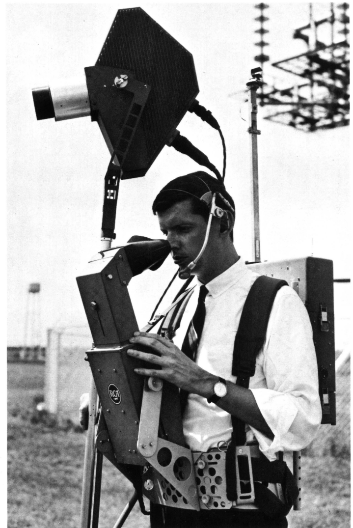
At RCA, development of a 56-pound portable color camera, suitable for use on moon surface, is an achievement expected to have profound influence on miniaturization of future television equipment.
