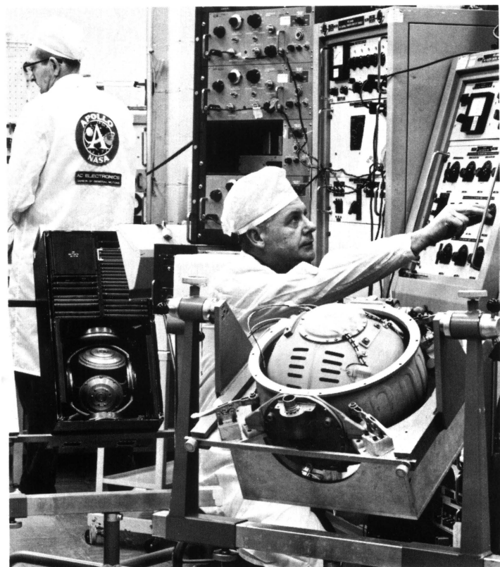
At AC Electronics, experience gained on Apollo guidance and navigation system, right, prepared the company for development of automatic inertial nav system, left foreground, for gigantic Boeing 747.
