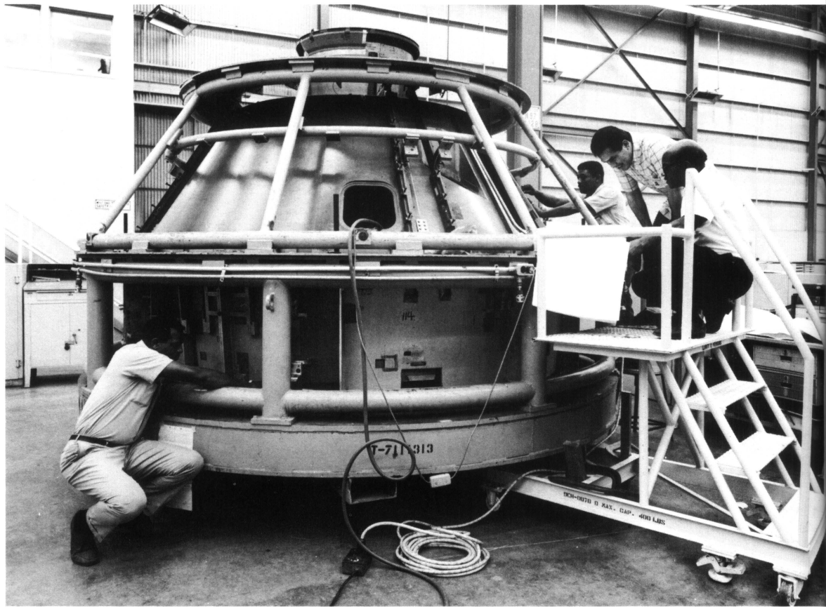
Cone-shaped primary structures for the AAP birds are virtually identical to Apollo. There are to be numerous changes inside the command and service modules.
