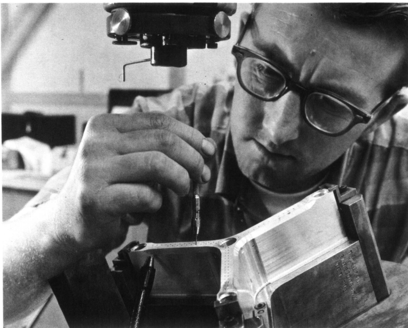
Modern manufacturing techniques, including electrical discharge machining, above, are used on engine injectors.
