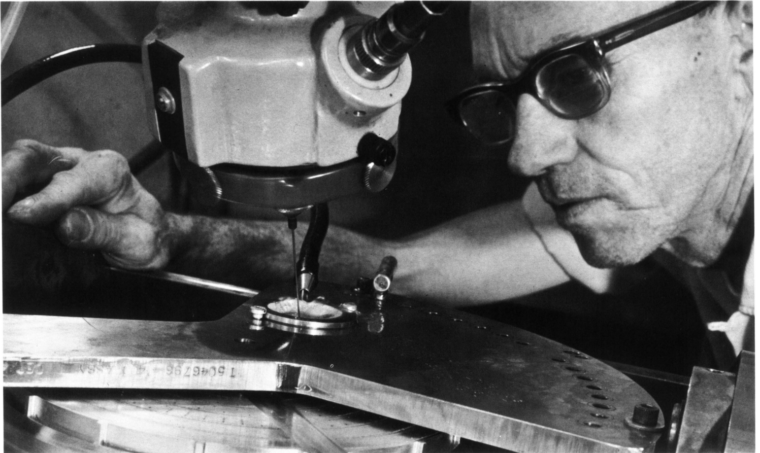
Modern manufacturing techniques, including electrical discharge machining, above, are used on engine injectors.
